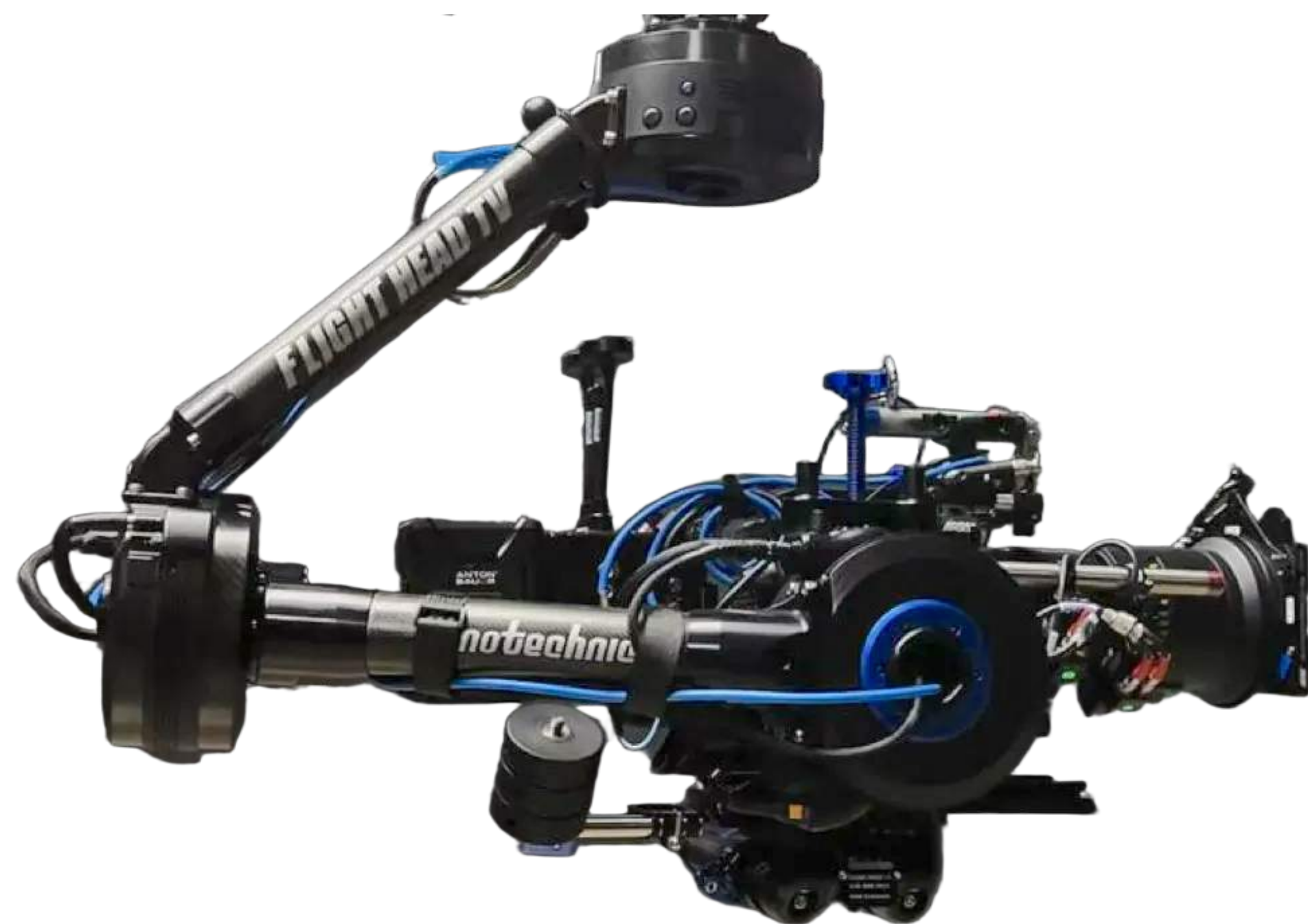
FLIGHT HEAD TV - head weight 13 kg, payload 15 kg, Roll/ Pan/Tilt \pm 360^\circ 3 turns, speed 120^\circ/\text{s}
