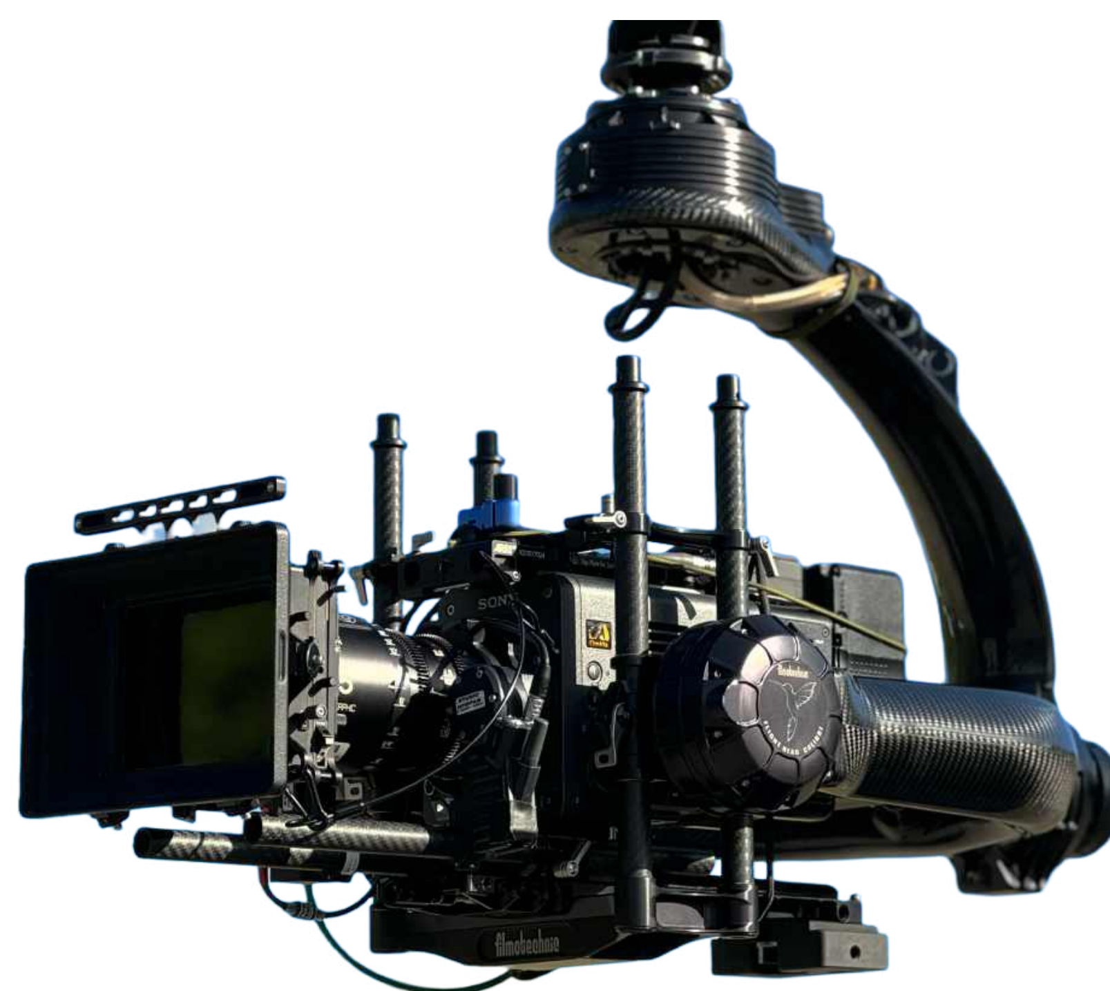
FLIGHT HEAD FALCON - weight 11 kg + Donut 2 kg, payload 34 kg, w. Donut FREE NODAL ROLL 360°, Pan/Tilt speed 120°/sec
